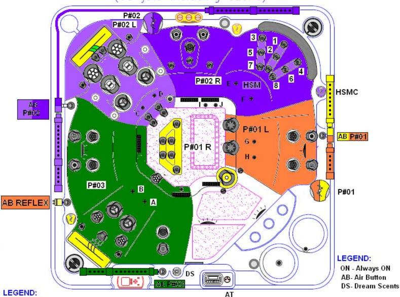
Pump no.1 is orange, yellow or shades of yellow Pump no.2 is purple or shades of purple Pump no.3 is green or shades of green HSM - HydroSequence Massage Seat HSMC - HydroSequence Massage Speed Control AT- Air Therapy; Air Jets (A,...,J)
