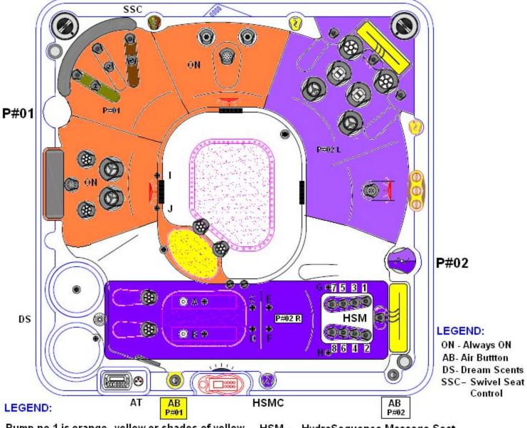
Pump no.1 is orange, yellow or shades of yellow Pump no.2 is purple or shades of purple HSM - HydroSequence Massage Seat HSMC - HydroSequence Massage Speed Control AT- Air Therapy; Air Jets (A,...,J)
