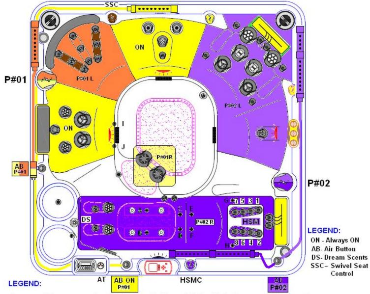
Pump no.1 is orange, yellow or shades of yellow Pump no.2 is purple or shades of purple HSM - HydroSequence Massage Seat HSMC - HydroSequence Massage Speed Control AT- Air Therapy; Air Jets (A....J)
